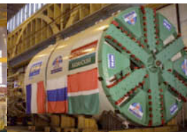
Soft ground TBM
