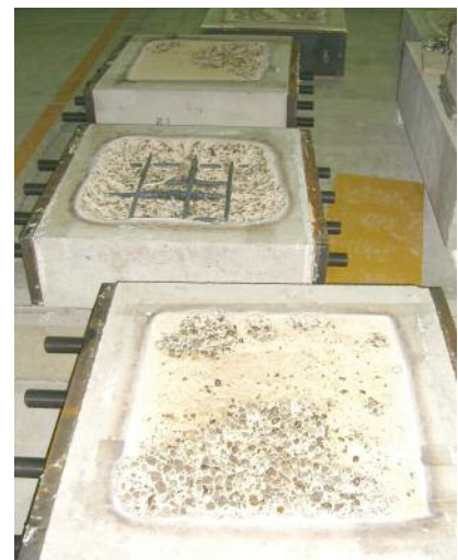
Right: Fig 1 - Concrete panels showing the spalling mechanism
