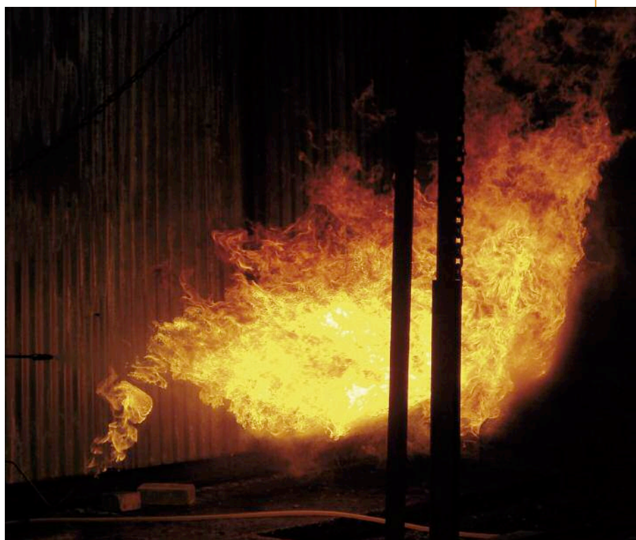
Right: Burning hydraulic fluid spray release
