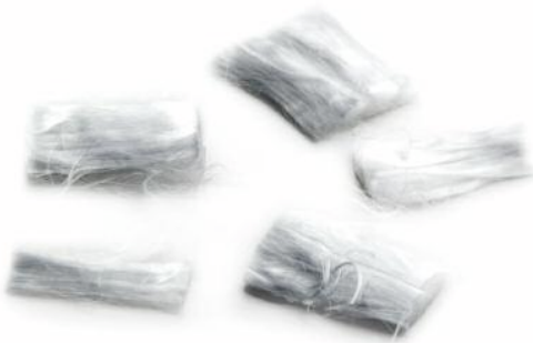
Above: Example of synthetic fibres used in protection against fire
