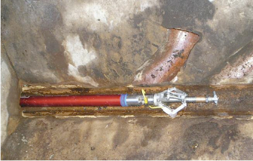
Left: The PipeTrack system for long run location surveys from within a pipe without need for surface access except at the end points. (picture courtesy of Infotec)
