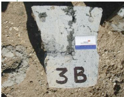
Above: Typical lattice girder shadow shotcrete trial
