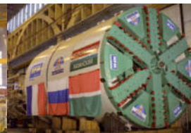
Soft ground TBM
