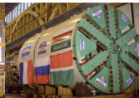
Soft ground TBM
