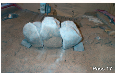
Above: Fig 7 - Characteristic fracturing of blocks embedded in soft sand grout
