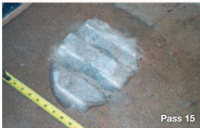
Above: Fig 9 - Chip formation of blocks embedded in a stiff matrix [7]
