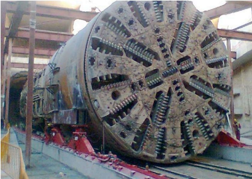
Above and right: The TBM sliding process underway in Sagrera shaft
