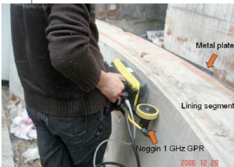
Above left: Fig 2 – EM wave velocity of the lining segments Right: Fig 3 – 1GHz data for the EM wave velocity test of the lining segments
