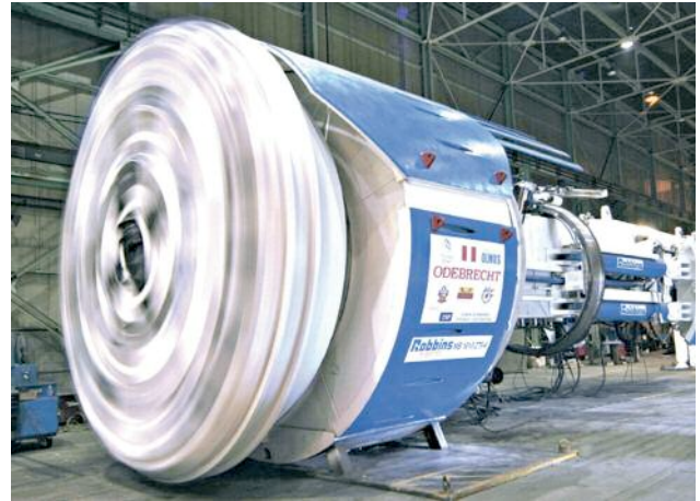
Above: The 5.3m diameter Robbins TBM assembly at Los Olmos, Peru; Right: The open shield was chosen due to high overburden
