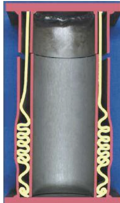
Above, left: Fig 4 – Load displacement diagram for a project designed group of 4 LSC (B Moritz 2008); Above, right: Section through a yielding element [7]
