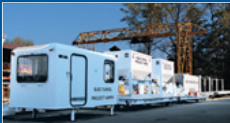
SRISAILAM TUNNEL, India JAIPRAKASH Ltd. men box, silo box, crane car, segment car, flat car
