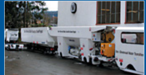
DEZ-GHOMROUD WATER TRANSITION TUNNEL, Iran SABIR Co. muck cars, mortar cars, segment cars, menrider
