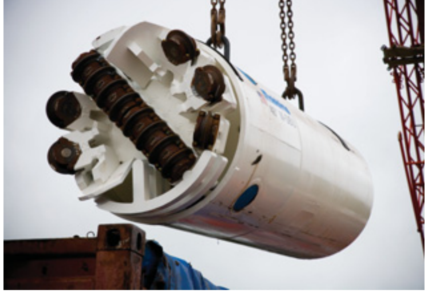
Above: A Robbins SBU-M utilises disc cutters to bore hard rock of over 170MPa
