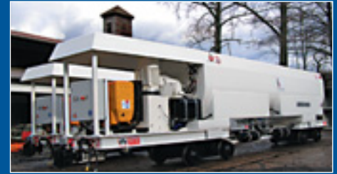
GAUTRAIN, South Africa Bombela Ltd. mortar cars, men boxes
