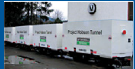
PROJECT HOBSON BAY TUNNEL, Australia McCONNEL Dowell Ltd. floorshaft cars, segment cars, flat cars
