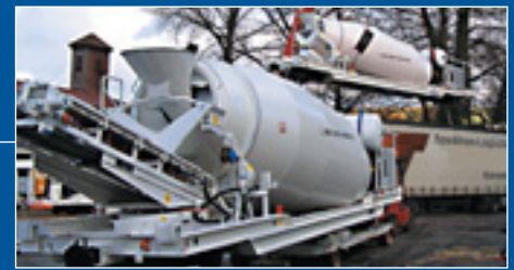
ARGE TUNNEL WIENERWALD, Austria PORR & BILFINGER BERGER rail running mixers 12/16 m 3
