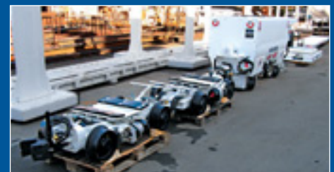
RENO CROSSING, Italy I.C.O.P. mortar cars, segment cars, flat cars
