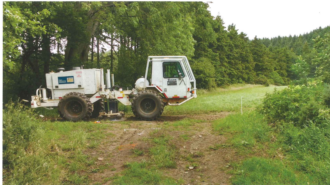
Above: Preparations for the Sirius Minerals MTS tunnel design (Yorkshire) included a programme of geotechnical drilling, in situ testing and seismic reflection surveys to characterise the geology to a depth exceeding 400 m
