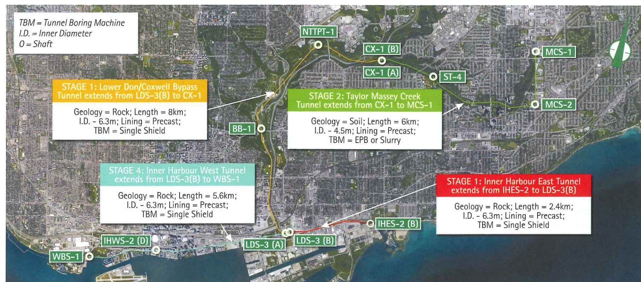
Above: Overview of tunnel stages 1, 2, and 4 for Toronto's DR&CW project
