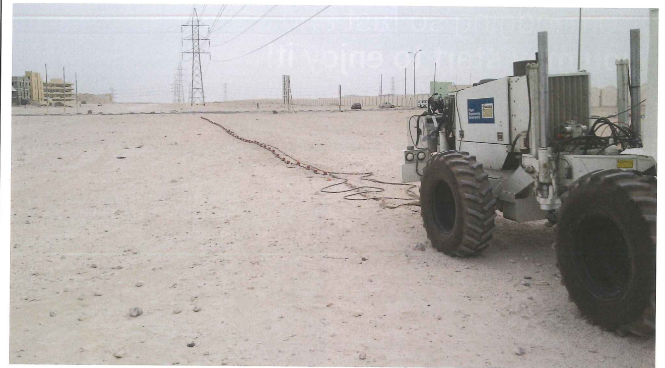
Above and below: High resolution seismic reflection surveys played a key role in the Doha Metro project in reducing the risk of tunnel boring machines encountering unforeseen cavities in the local strata
