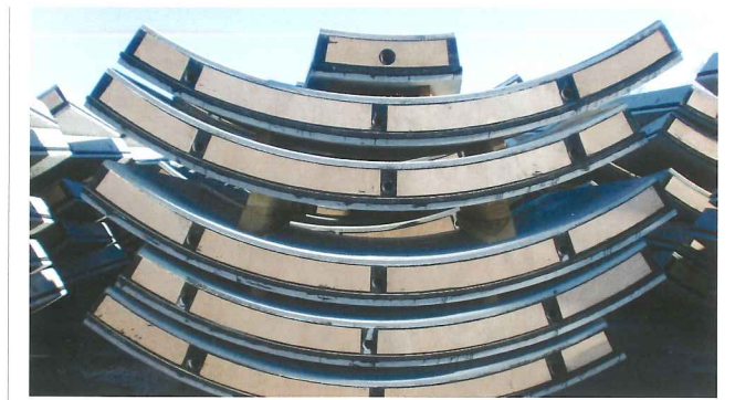
Above: Segments stacking for storage and schematics of forces acting on bottom segment
