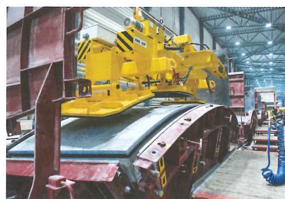
Above left: The SR99 project Centre: A casting yard in Beijing Above right: Demoulding segments for the Follo Line
