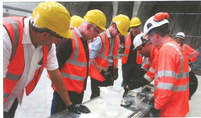
Above: Delegates at the BASF Underground Construction workshop test the properties of spray applied waterproof membrane
