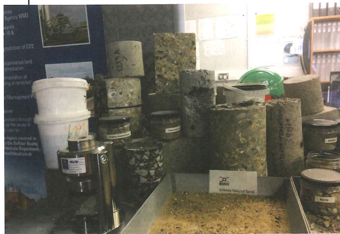
Below: Concrete core samples in the Materials Testing Laboratory
