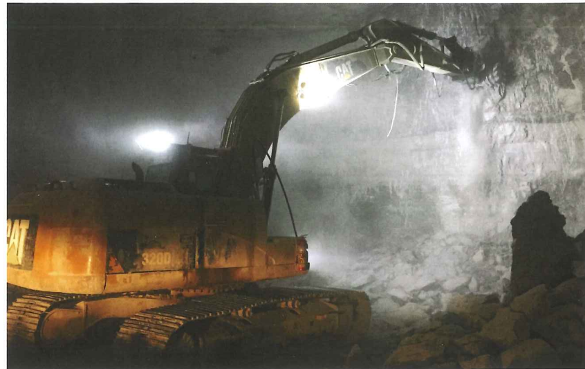
Above: An Alpine Rockwheel model D30 (110-kW) installed on a CAT320 excavator
