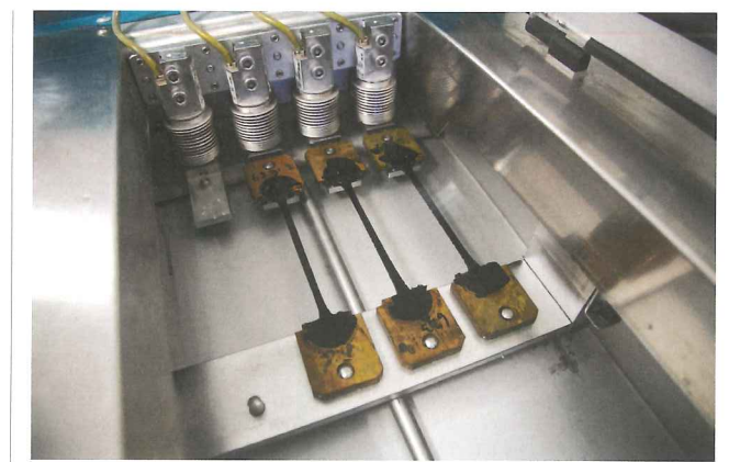
Above: A bitumen sample is stretched in the laboratory for force ductility measurement
