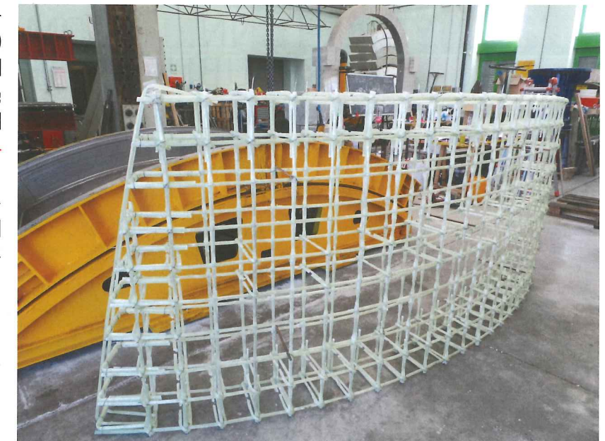
GFRP REINFORCEMENT MADE BY ATP AT THE LABORATORIES OF THE UNIVERSITY OF ROME BEFORE BEING TESTED
