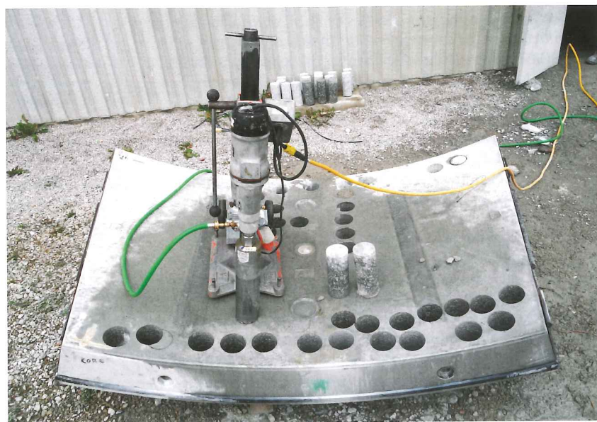
Above: The coring process and cores
