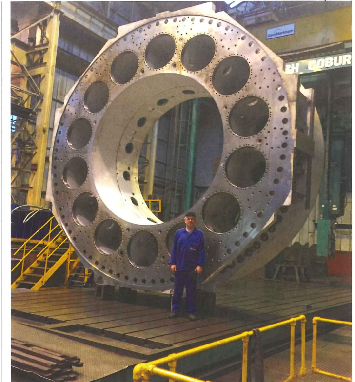
Above: Bearing housing manufactured for NFM
