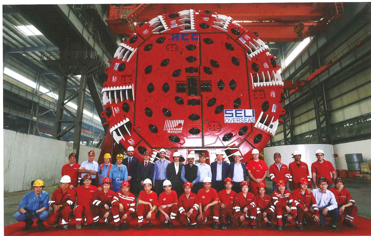
The TBM will now be disassembled and shipped out to the site in northern India to bore a low pressure headrace tunnel
