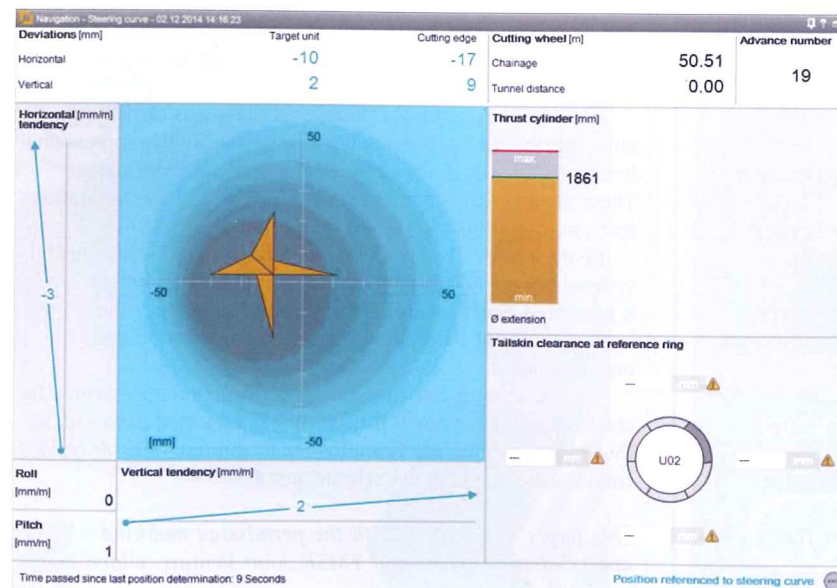
Below: Figure 3, Software system for control of deviations by setting a steering curve during TBM progression
