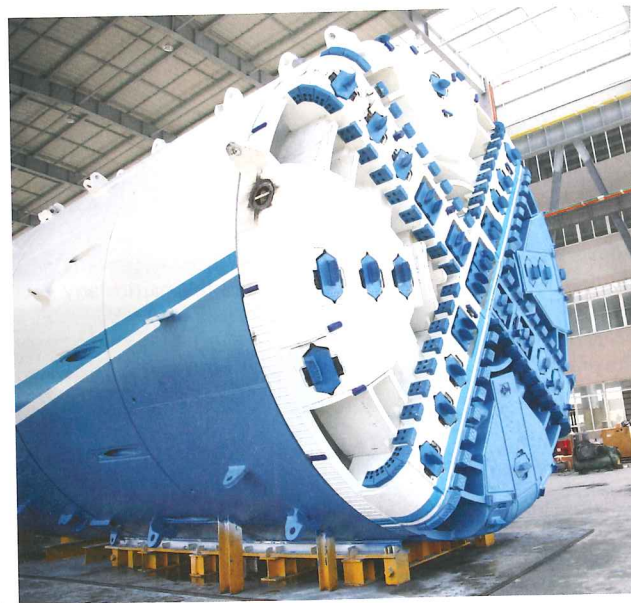
Above: An EPBM undergoing factory acceptance
