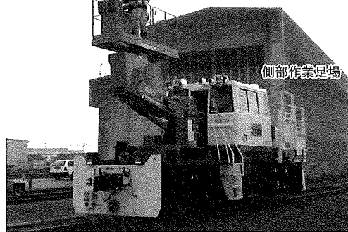
STARS ( Shinkansen Tunnel Aseismic Repair Staging-car )
