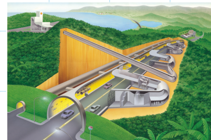
Tunnel Ventilation System
