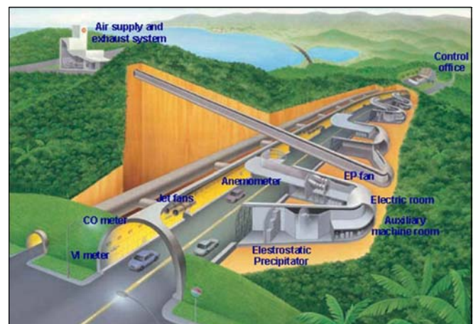
Fig. 2 Tunnel Ventilation System
